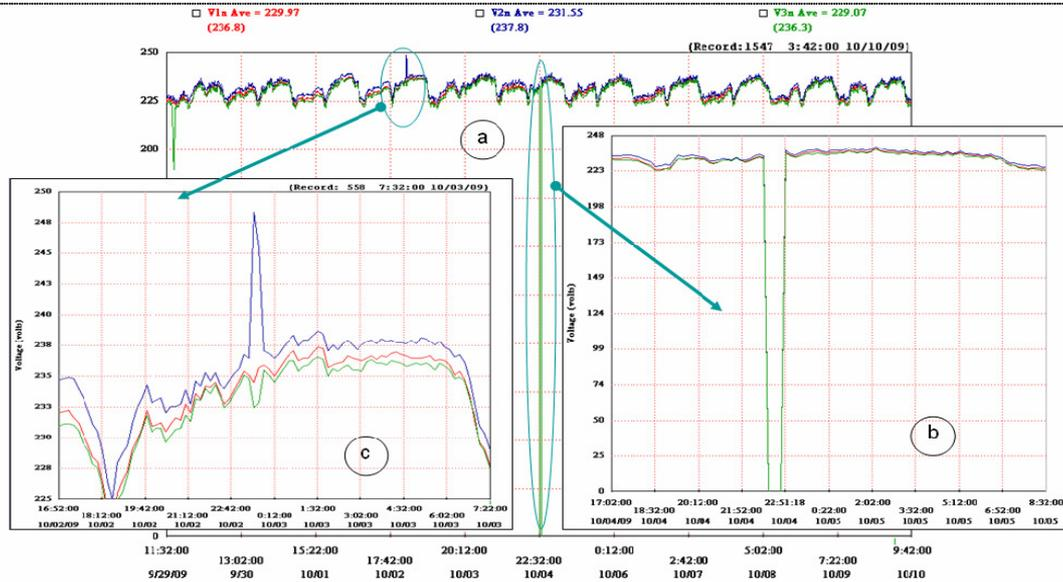
FIGURE 3. A VOLTAGE DIP SITUATION
