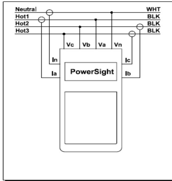
FIGURE 2. THREE PHASE RMS VOLTAGE PROFILE DURING MONITORING PROCESS A) COMPLETE PLOT OF MONITORING PROCESS B) SITUATION OF SUSTAIN INTERRUPTION VOLTAGE C) SITUATION OF AN OVERVOLTAGE INSTRUMENT CONNECTION FOR UNBALANCED LOADS
