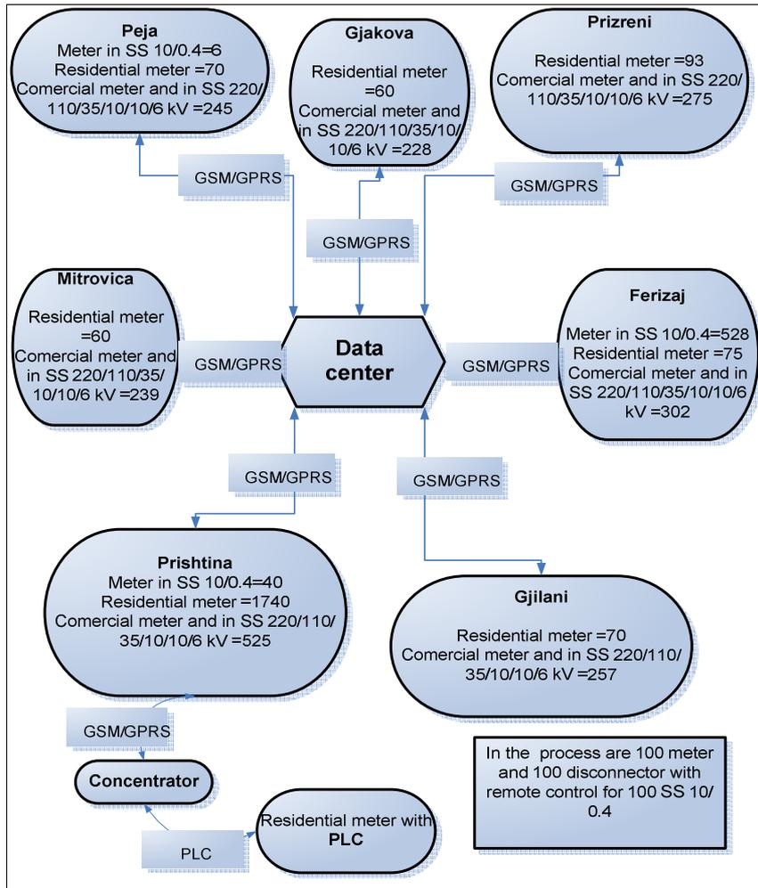
FIGURE 3. COMMUNICATION OF WITH SMART METERS WITH REMOTE READING CENTRE
